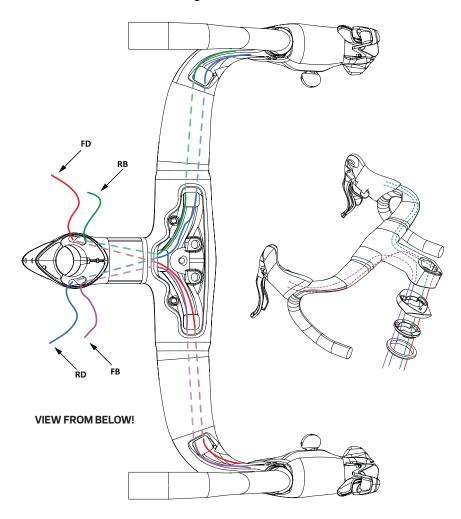
ATTENTION! The stem exit hole on the right-hand side the RB hose must be in front of the FD housing.
