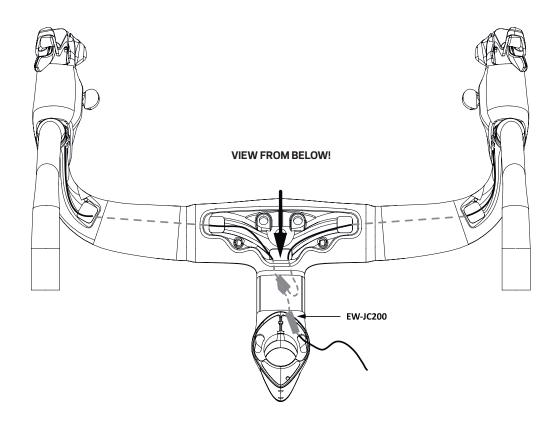
9.4 Install the handlebar on the steering tube. The lower support surface of the handlebar must be at X+2 cm away from the upper planar surface of the top cap. Where X is total height of the spacers you are going to install (e.g. if you install 3 cm of spacer, you must place the adapter at 5 cm away). This way you will have enough space to route the cables and assemble the spacers. Refer to chapter "12. HEADSET ADJUSTING" for more details about spacers.
