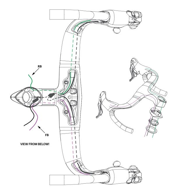
ATTENTION! The stem exit hole on the left-hand side the FB hose must be in front of the Di2 wire.
