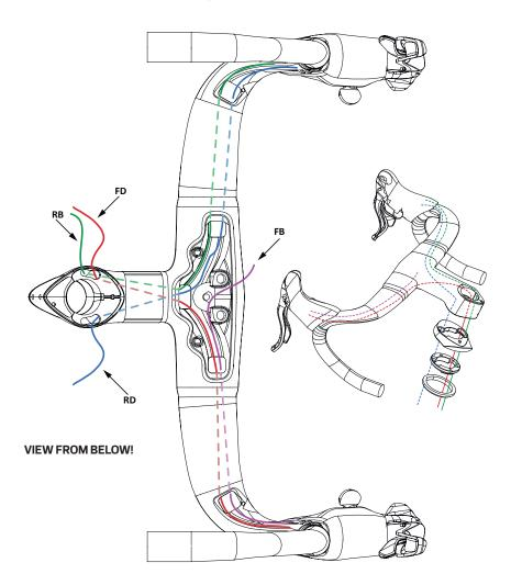
ATTENTION! In the stem exit hole on the right-hand side the FD housing must be in front of the RB housing.
