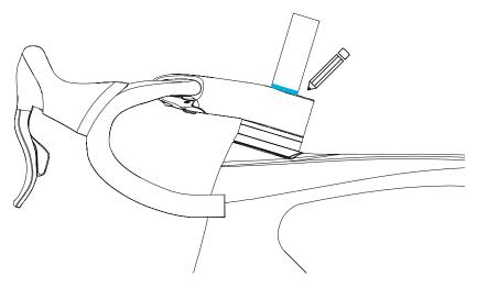
If you intend to leave the steerer tube longer above the stem (in order to maintain the possibility to rise the handlebar at a later date), place the desired number of standard aero spacers (not split) above the stem, as illustrated below, and mark a line just as described along the top edge of the upper spacer.
