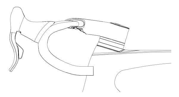
ATTENTION! The split spacers have larger dimensions than usual because of having to fit with the 1" ½ upper bearing. So, they cannot be used on the upper side of the handlebar. For the upper side, the standard aero spacers must be used (see also paragraph 12.4).
